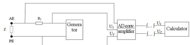
Fig. 1 — Structural chart of impedance meter.
