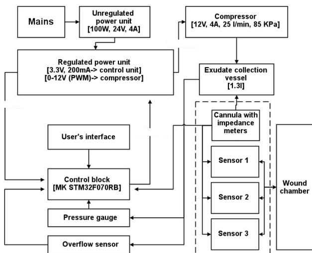
Fig. 2 — Structural diagram of the aspirator pump under development.
