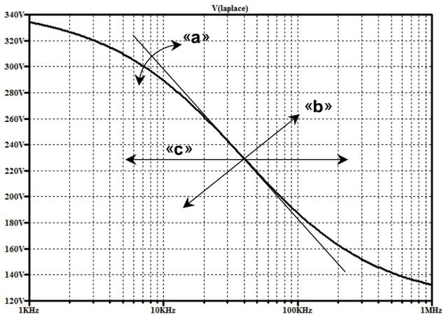
Fig. 8: The frequency dependence graph for the final equivalent circuit based on the Laplasian operator for the porcine muscle tissue simulating with indication of the adjusting factors effect direction
