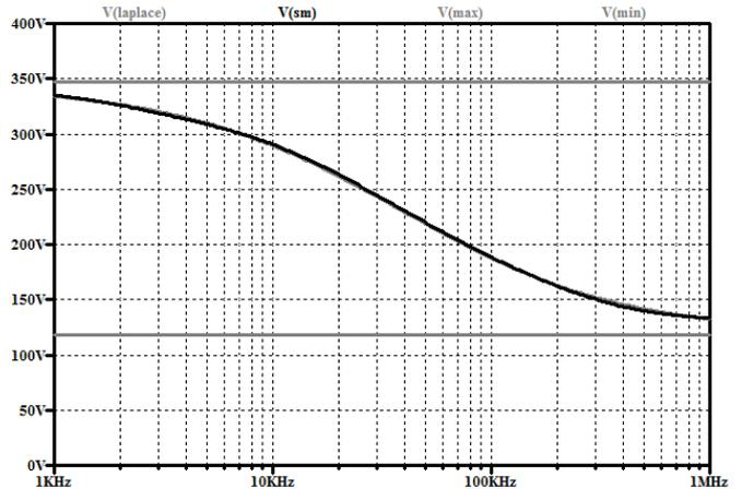
Fig. 6: Frequency dependence graphs for the final variant of the equivalent circuit based on the Laplasian operator and the semi-segment series RC equivalent circuit indicated within the "Rmax" and "Rmin" limits for the porcine muscle
