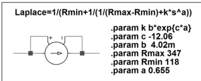
Fig. 7: Final variant of the equivalent circuit based on the Laplasian operator and adjusting parameters of the biological tissue sample for the porcine muscle tissue
