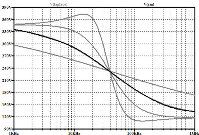
Fig. 5: Frequency dependence graphs for the Laplasian operator-based modification of (a number of gray graphs) and the semi-segment series RC equivalent circuit (black graph).
