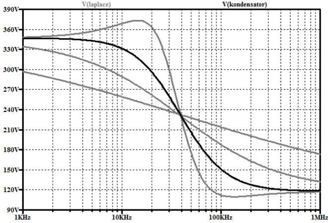
Fig. 4: Frequency dependence graphs for the Laplasian operator-based modification of (a number of gray graphs) and initial (black graph) simple equivalent circuit developed for simulating the porcine muscle tissue sample
