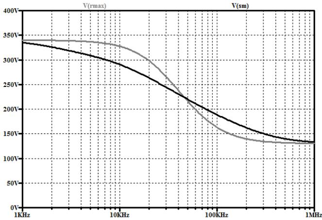
Fig. 2: Porcine muscle biological tissue impedance function of the simple equivalent circuit simulation result at the frequency range of 1 kHz to 1 MHz. The equivalent resistance in Ohm/V is marked along the Y-axis, and the measured voltage frequency in Hz is marked along the X-axis. The measured characteristics is represented in black, and the result of the simple equivalent circuit simulation is shown in gray
