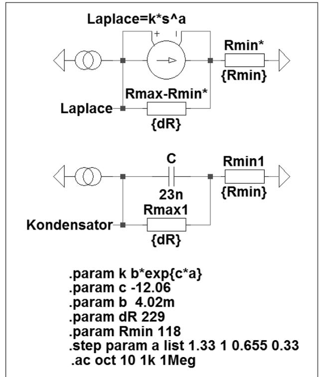
Fig. 3: Modified based on the Laplasian operator (on top) and the initial (below) variants of the simple equivalent circuit with a step-based changing derivative order for the porcine muscle tissue sample
